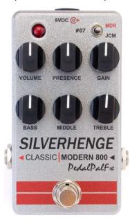
Thanks to the three way toggle switch, we add to this reissue some of our favorite mods in the 800 series, like the Mod #07 related to the gain voicing switch and the Mod MDR that adds more saturation into the circuit delivering a modern JCM800 sound, similar to the ones you can get from the PAL800-V3 GOLD Overdrive.
